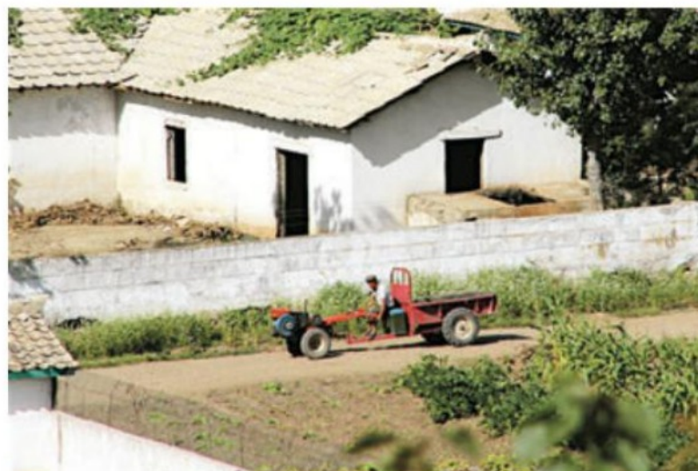
1.22 Originally developed from mechanised ploughs, the simple Chinese-made walking tractor is an example of low cost technology used on many farms in East, North-east and South-east Asia. This example is on a collective farm near Sariwon, North Korea.
